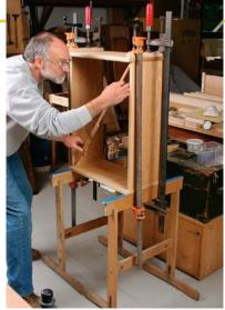
**Hold it up and hold it fast.** The design creates a convenient clamping surface, with the top stretcher acting as a caul.
