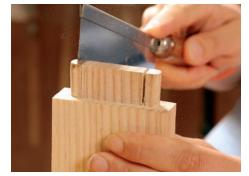
**Finish them at the bench.** Use a chisel and file (top) to shape the tenon ends to match the routed mortises. A pair of handsawn kerfs (above) will make room for the wedges.
