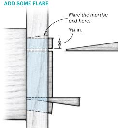
**Room to spread.** These through-tenons are wedged for strength and a decorative touch. Flare the mortise ends with a rounded file so the tenons can spread as you drive the wedges home.
