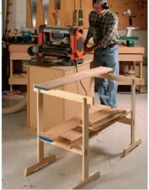
**Beasts of burden.** The lower stretchers provide an additional rack for lumber storage either long-term or during work.
