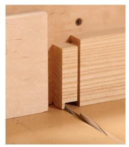
**Start tenons on the tablesaw.** Use a crosscut sled with a stop to cut the shoulders and nibble away the ends (above). A tenoning jig (right) makes quick work of the cheeks.
